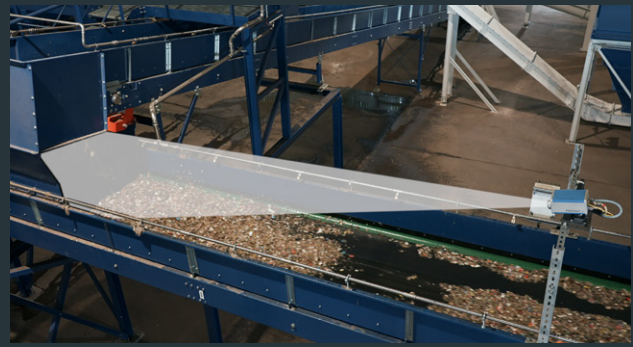
PYROsmart® one always keeps belt transfer points in view and detects critical temperatures in free-falling material.
