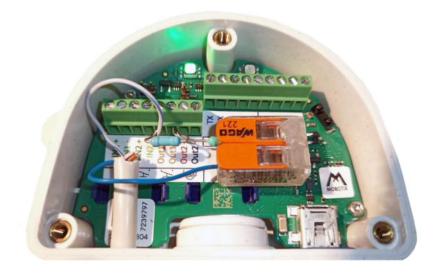
This box is installed on the camera side and connected to the M73 camera via the USB interface.
