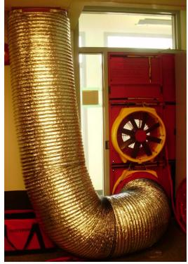
Now, the EPA, IRI, FM, other insurers, fire suppression equipment manufacturers, and the FSSA all encourage door fan tests on every installation. Door Fan tests should be repeated annually or whenever extra holes are made in the enclosure.
