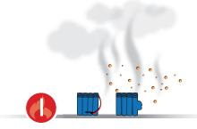
When Lithium-ion batteries are exposed to heat, physical/impact damage or over charging they go into thermal runaway.
