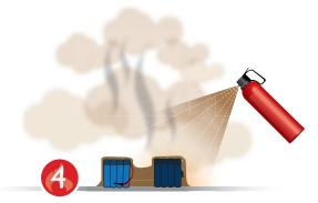
AVD is applied as a fine mist, which instantly cools the batteries and extinguishes the flames.
