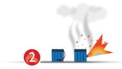
The cells are sufficiently swollen releasing hot flammable gases (hydrocarbons) which can ignite.
