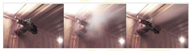
By monitoring the pressure in the pressure cylinder, the test container and also the position of the blast vent blades at 20HZ, the relationship between the rates of gas volume increase in the test container, verses the rate at which the blast vent blades open, can be associated with the peak pressure in the container.
