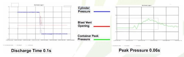
The data collected from the AFP live discharge tests can also be integrated into the results produced by certain software simulations.
