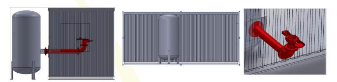
This produces the same instant pressure discharge as can be produced during a switchgear fault, with a typical total discharge time of between 0.1 and 0.2 seconds. When the correct sized AFP SHX UN Blast vents are installed, this results in the time to peak pressure, in the building, being suppressed to just 0.06 seconds which has the effect of massively reducing any potential overpressure that could result in structural damage.
