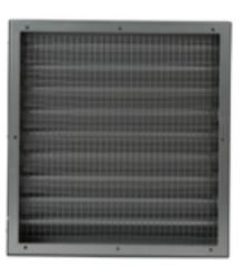
The EXP Exterior Louvre unit is used with AFP's DUX range of pressure relief vents in halocarbon installations. It has been specifically designed to provide a Free Vent Area (FVA) matching that of DUX while providing the weather protection essential for two-way vents in exterior walls.
