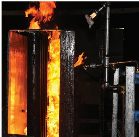
To enhance the fire suppression capability of the two individual agents, a single control device delivers both CAF and CAF mist to the fire through separate nozzles that are positioned to deliver foam and foam mist in one integrated stream.
