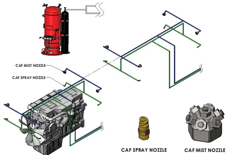
components into the creation of a single more effective suppression system. This, in tandem with state of the art system components and fire detection make for a highly advanced, very effective fire suppression system.
