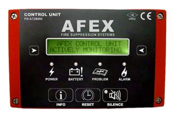
CONTROL UNIT HARNESSES - A729200 BASIC HARNESS / A729400 ADVANCED HARNESS The Control Unit harness connects the Control Unit to the fire suppression system's detection and actuation circuit(s), the external power circuit, and the external alarm/problem signaling device (A729400 harness only). Automotive type electrical connectors are included with the harnesses.
