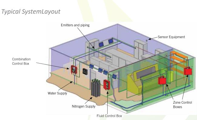
Dry Contact Vortex Combination can also be used for Multi Zone System Applications
