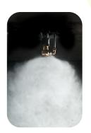
Patent 7,686,093 - Dual Extinguishment fire suppression system using high velocity low pressure emitters. Foreign patents also applied for and granted .
