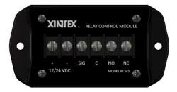
The RCM5 has a 6 position terminal strip located on the top face of the unit. Power must be supplied to the unit, as well as the signal from a Xintex detection device. When the RCM5 receives the signal from the connected Xintex device, the relay is tripped. The RCM5 can be used to interrupt a device's ground and disable the device.
