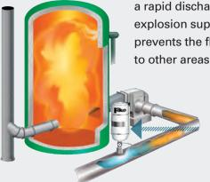
a rapid discharge of a chemical explosion suppressant which prevents the flame from spreading to other areas of the process system.
