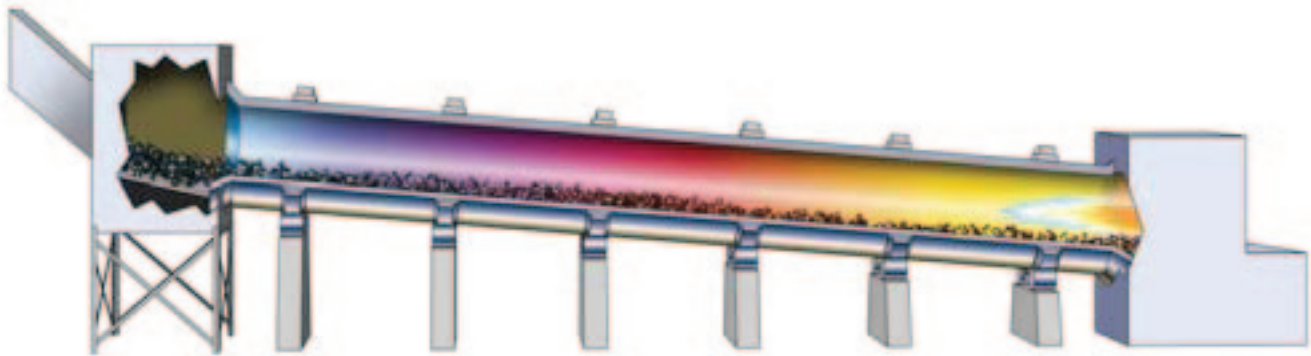
Figure 1: Typical Cross-Sectional View of a Cement Kiln
