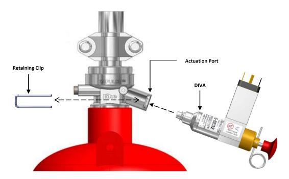
**WARNING:** Do not attempt to install the DIVA with the firing pin in the activated (extended) position.
