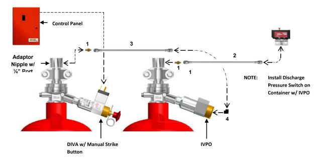
1<sup>st</sup> remove the 1/8" NPT Plug from Adaptor Nipple, then install Actuation System as shown above. Secure Actuation tubing to a solid surface. Anchoring into plaster, sheetrock wall or any other facing material is NOT acceptable. For additional information regarding the installation and resetting of the IVPO, refer to the IVPO Component Spec (p/n 06-698-1-3).
