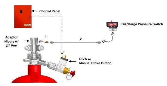
**EXAMPLE 2: ELECTRIC & PNEUMATIC ACTUATION – TWO CONTAINER SYSTEM W/ DIVA & IVPO**
