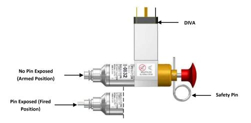
Install the wire lead w/ connector (Item no. 3) to the DIVA (Item no. 1) connector and secure with set screw.
