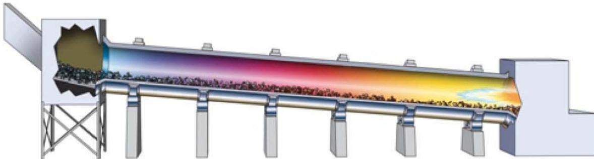
**Figure 1: Typical Cross-Sectional View of a Cement Kiln**
