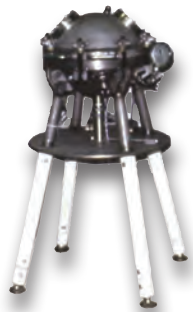
20-Liter Vessel – Used for K_{ST} and P_{MAX} determination
