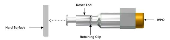
Remove Retaining Clip, IVPO is reset and ready to be installed on Impulse Valve.
